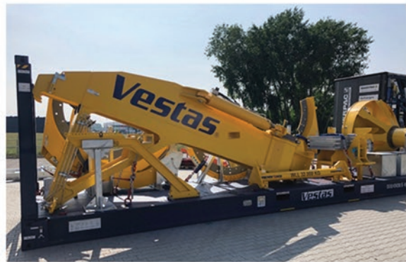
CakeBoxx 40ft special application Flat Rack for wind components, including customer-defined fitments for different cargos
