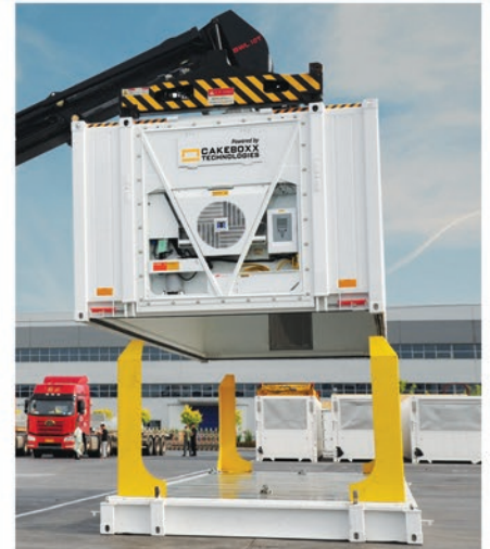
12' wide refrigerated CakeBoxx two-piece container for special temperature sensitive equipment
