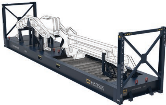
CakeBoxx 40ft special application Flat Rack for wind components, including customer-defined fitments for different cargos
