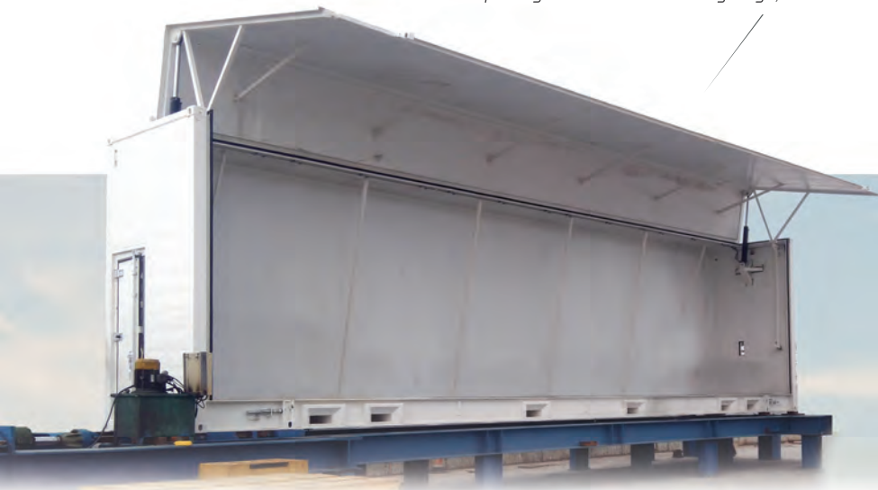
Side-opening container for loading large, sensitive cargos
