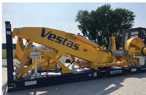
CakeBoxx 40ft special application Flat Rack for wind components, including custom fitments for different cargos
